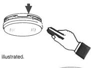
iii. Unclip and slide alarm as illustrated.
